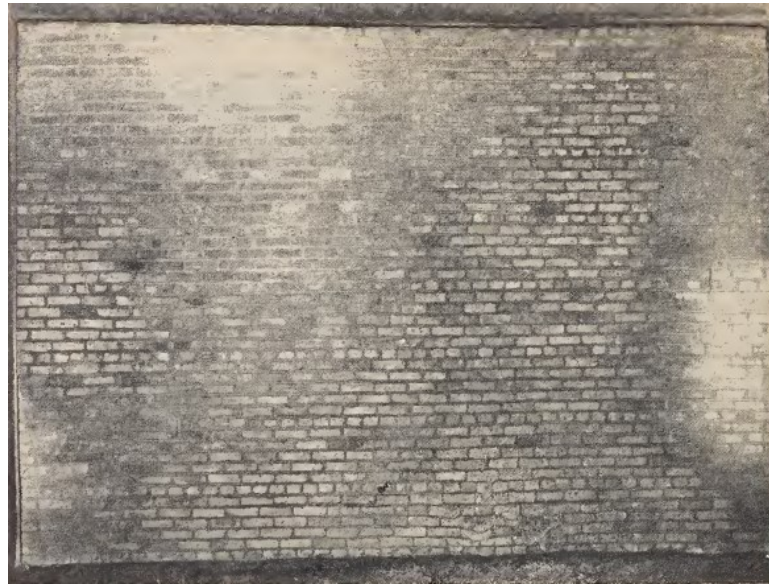
Fire exposed face of 205 mm concrete brick wall after 6 hr fire test
