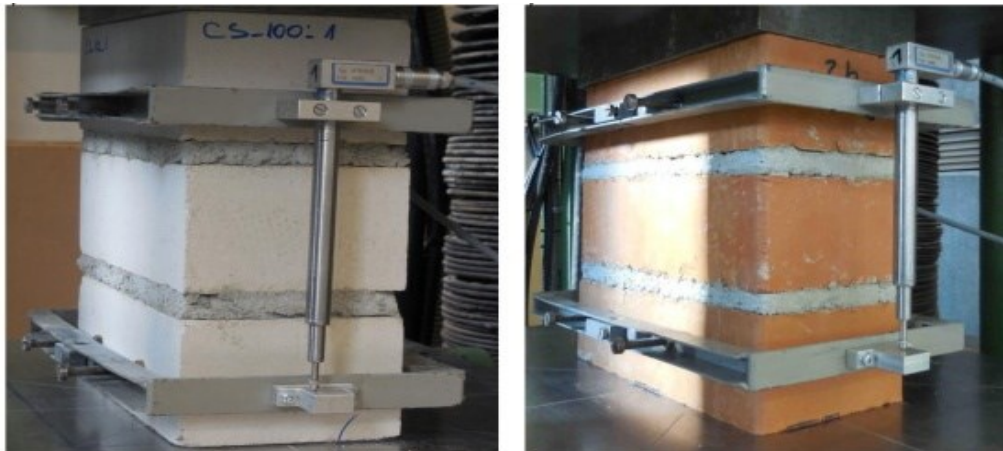
Fig. 6 Brick prisms under compression strength test (note: Left – calcium silicate brick prism, Right – clay brick prism) (Credit line: Elsevier, Construction and Building Materials, Experimental and numerical studies on masonry after exposure to elevated temperatures, Josipa Bošnjak, Serena Gambarelli, Akanshu Sharma, Amra Mešković, January 10, 2020, License Number: 4954620364144)
