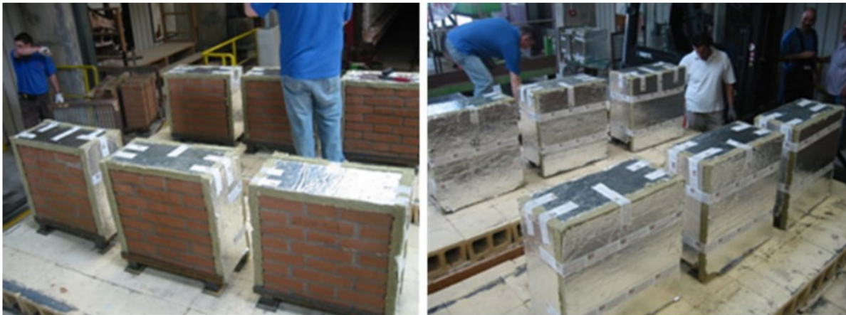
Fig. 11 Wallettes specimens to be put to fire tests as per [45] (Credit line: Springer Nature, Experimental Mechanics, Experimental and Theoretical Investigation on Masonry after High Temperature Exposure, S. Russo et al., April 21, 2011, License Number: 4954640044417)
