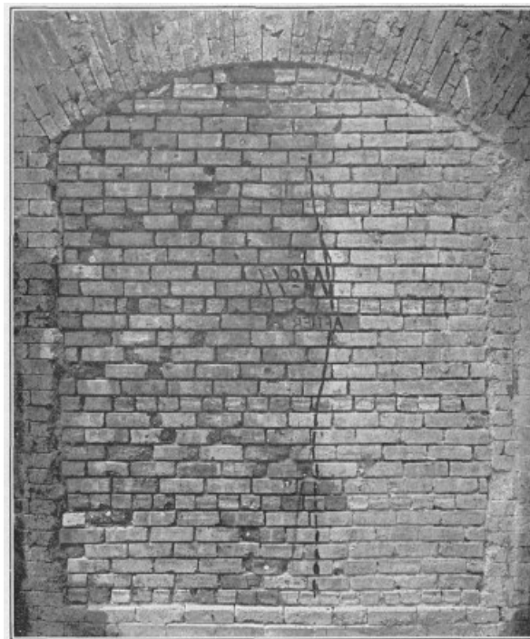
Face of Panel 11, Common bricks after fire test and quenching.
