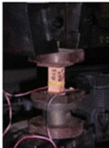
Fig. 5 Residual (post-heating) testing of masonry units by Russo et al. [45] (Credit line: Springer Nature, Experimental Mechanics, Experimental and Theoretical Investigation on Masonry after High Temperature Exposure, S. Russo et al., April 21, 2011, License Number: 4954640044417)
