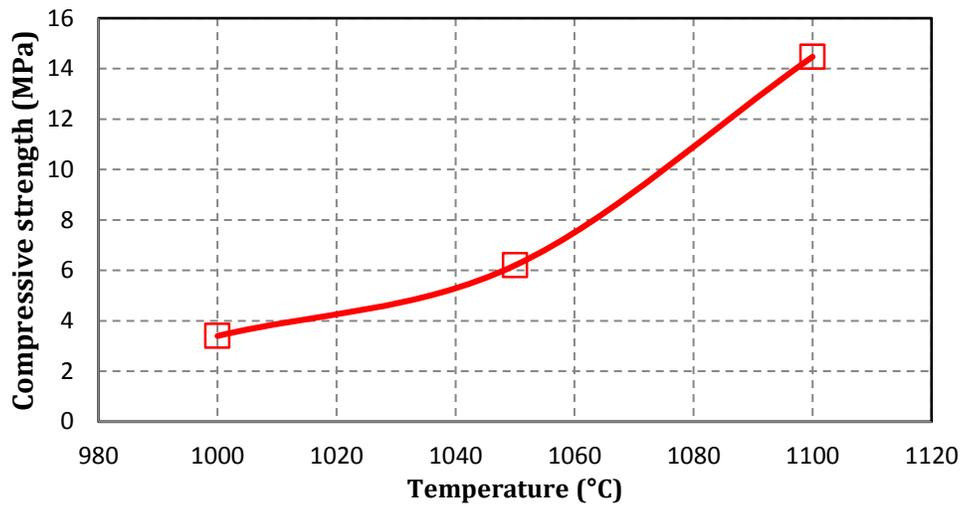
(a) Effect of sintering temperature
