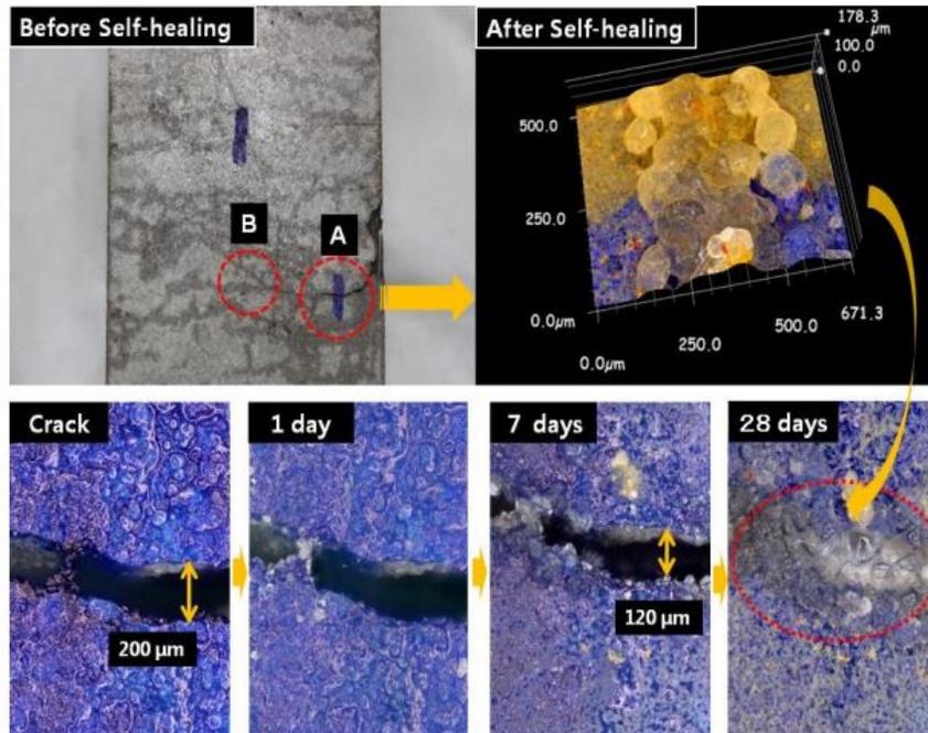
Fig. 22 Process of self-healing in concrete [264]
