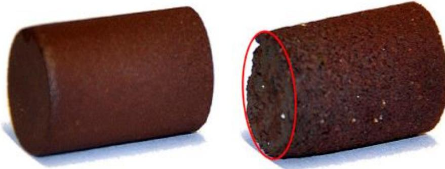
(a) Photograph of samples fabricated by Indyk and Benaroya [147], (left) is 1.44% porosity and (right) is 11.78% porosity
