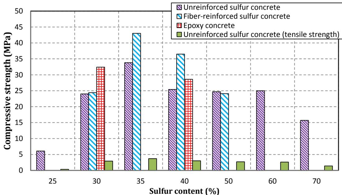
Fig. 17 Average compressive strength of various concretes tested in experiments by Omar and Issa [235,236]
