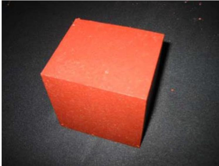
Fig. 34 Martian brick made by cold pressing [394] (Note: each side = 100 mm)
