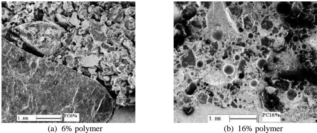
Fig. 16 SEM observations of two polymer concretes with varying polymer content [218]
