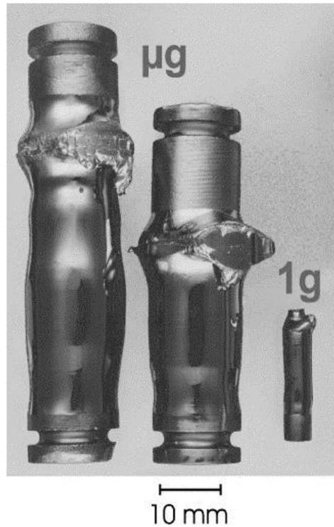
Fig. 27 Crystals grown in space under microgravity ( $\mu\text{g}$ ) (left and center) and on Earth under normal gravity (1g) (right) [358]
