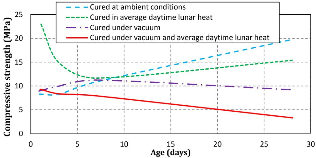
(a) Compressive strength of concrete under various curing conditions.
