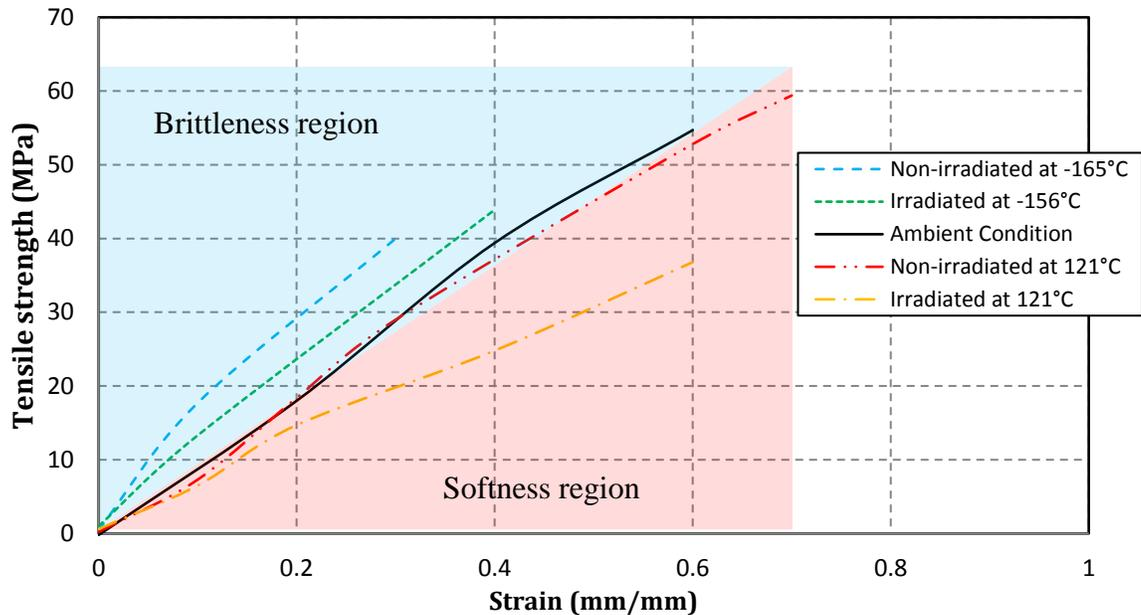
Fig. 25 Effect of radiation and temperature on tensile behavior of T300/934 graphite-epoxy composite [320]
