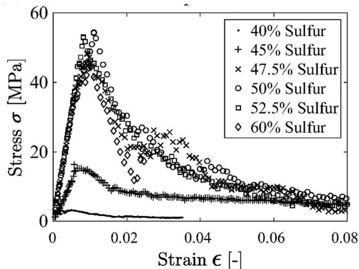
(a) Comparison of compressive stress-strain response for Martian concretes with various sulfur ratios
