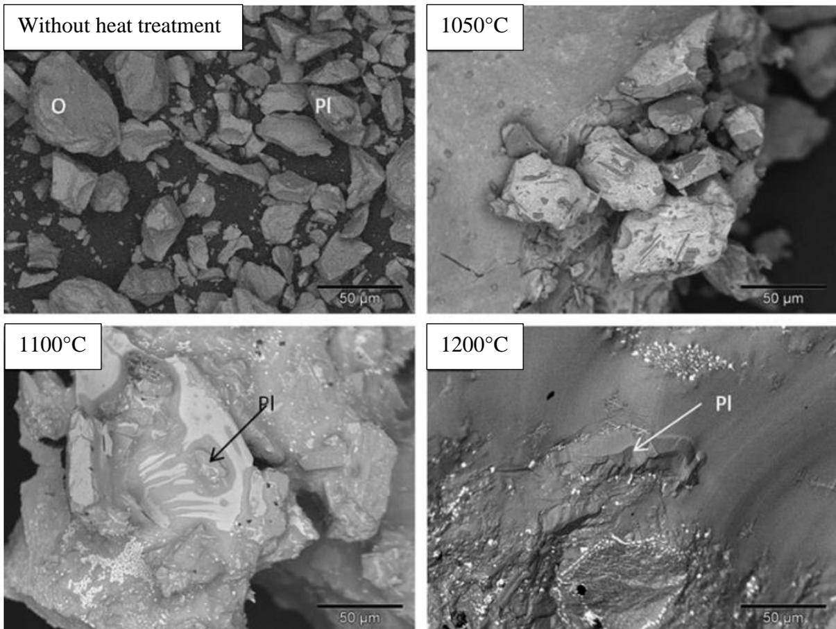
(b) Simulant JSC-1A after ambient condition; at 1050°C; at 1100°C; at 1200°C; individual particles are labeled Pl for plagioclase, O for olivine, and Py for pyroxene (Courtesy of NASA) – scale = 50 µm.
