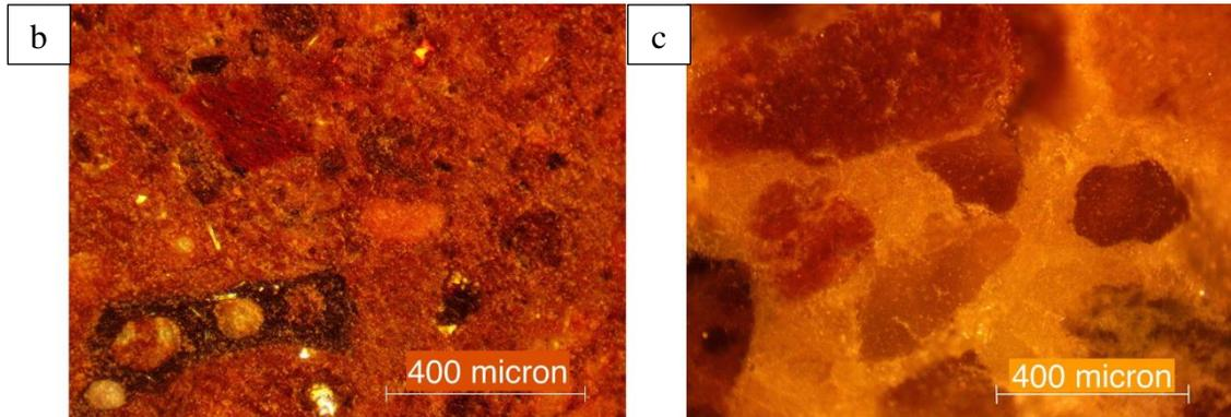
Fig. 19 Microscopic imagery of sulfur concrete with compositions of (b) 50% sulfur and 50% Martian soil simulant (c) 25% sulfur and 75% regular sand and a maximum particle size of 1 mm. [243]
