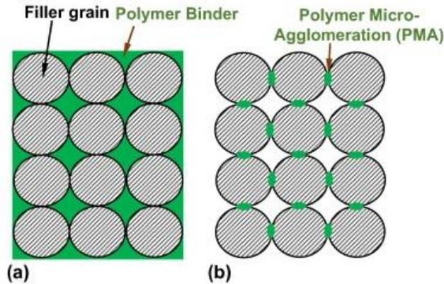
Fig. 26 Illustration of (a) close-packed grains filled by  $\sim 8.6$  wt.% binder; and (b) polymer micro-agglomerations (PMA) that only bridges filler grains [317]
