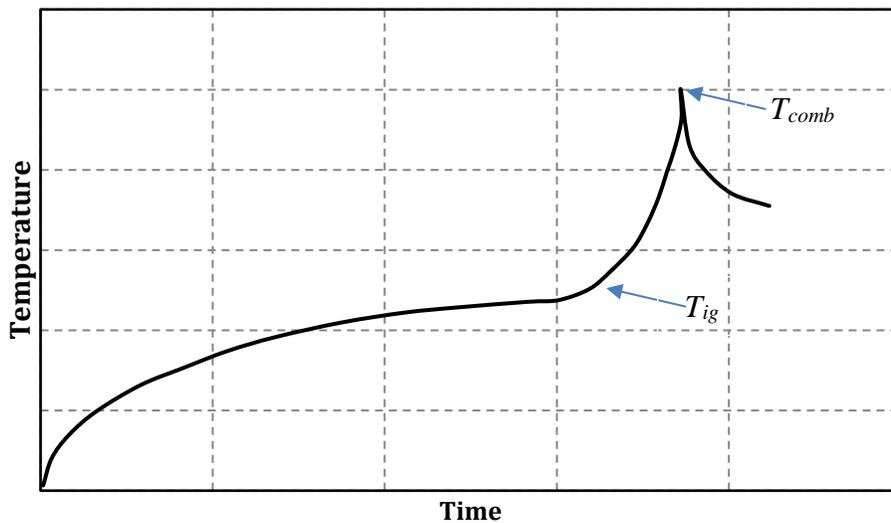
Fig. 30 Typical temperature-time history of combustion process
