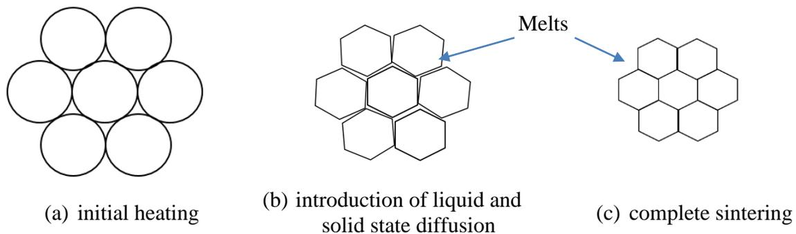
Fig. 28 Illustration of sintering process
