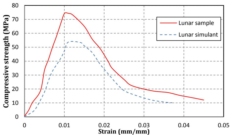
Fig. 14 Measured stress-strain response of concrete samples tested by Lin et al. [196]
