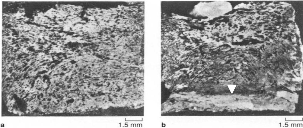
Fig. 31 Microstructures of products reacted (a) under microgravity conditions and (b) under normal gravity conditions (Downward arrow shows increase in aluminum segregation) [384]
