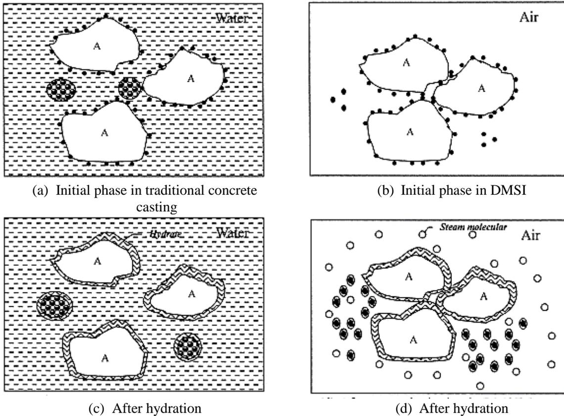
Fig. 32 Schematic of hydrates for traditional and DMSI process [386]
