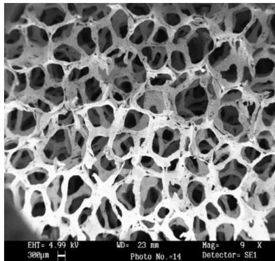
Fig. 24 SEM image of typical metal foam [305]
