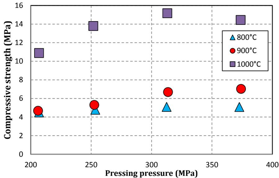
Fig. 35 Compressive strength of simulated lunar soil under varying conditions [398]
