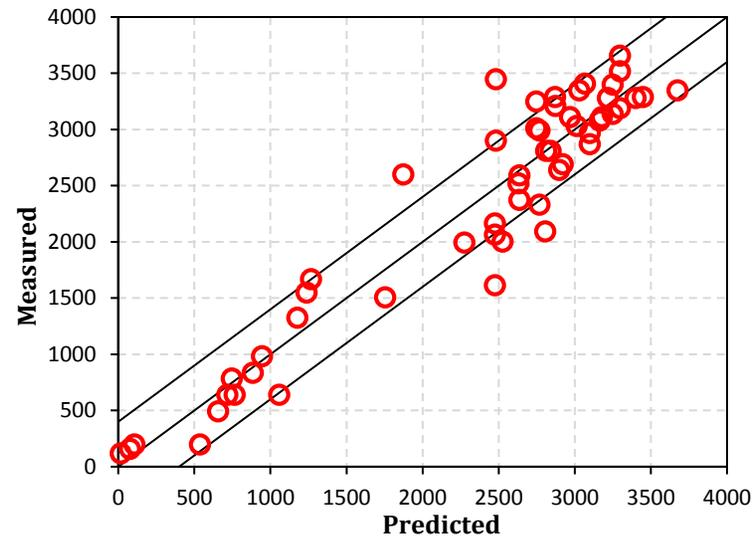
(e) Residual capacity of columns (in kN)
