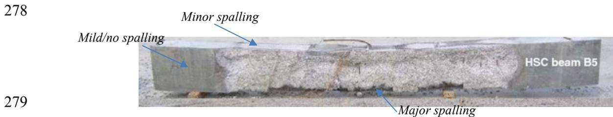
280 Fig. 4 Demonstration of magnitude of spalling used in training the developed CV model –
