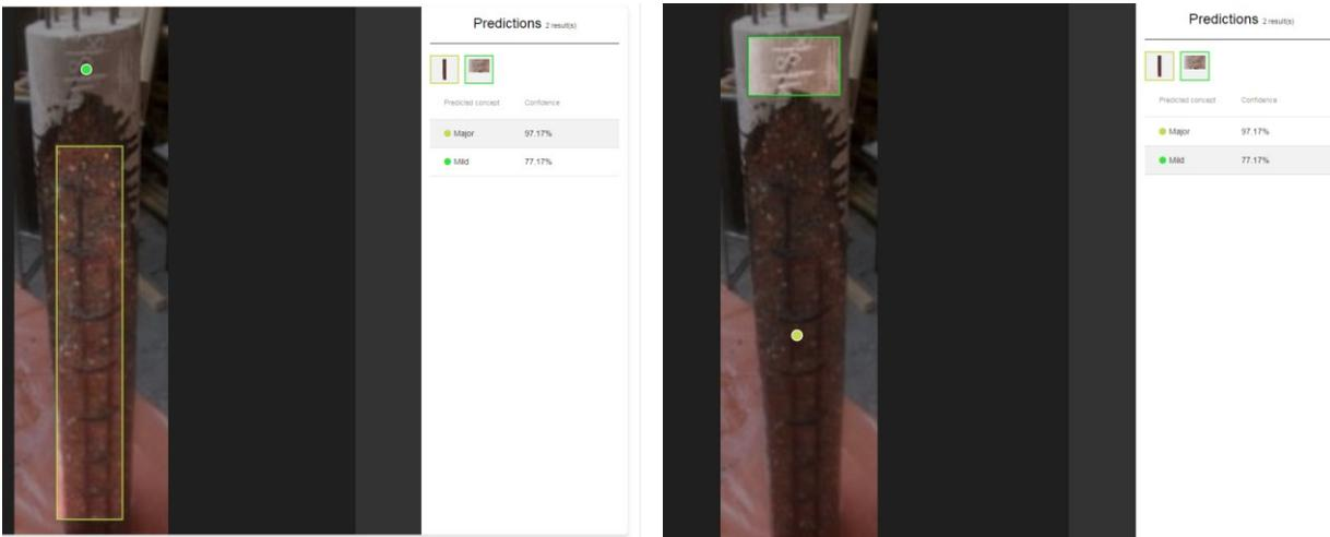
404 Fig. 7 Detection of magnitude of spalling through CV analysis (bottom images taken from
