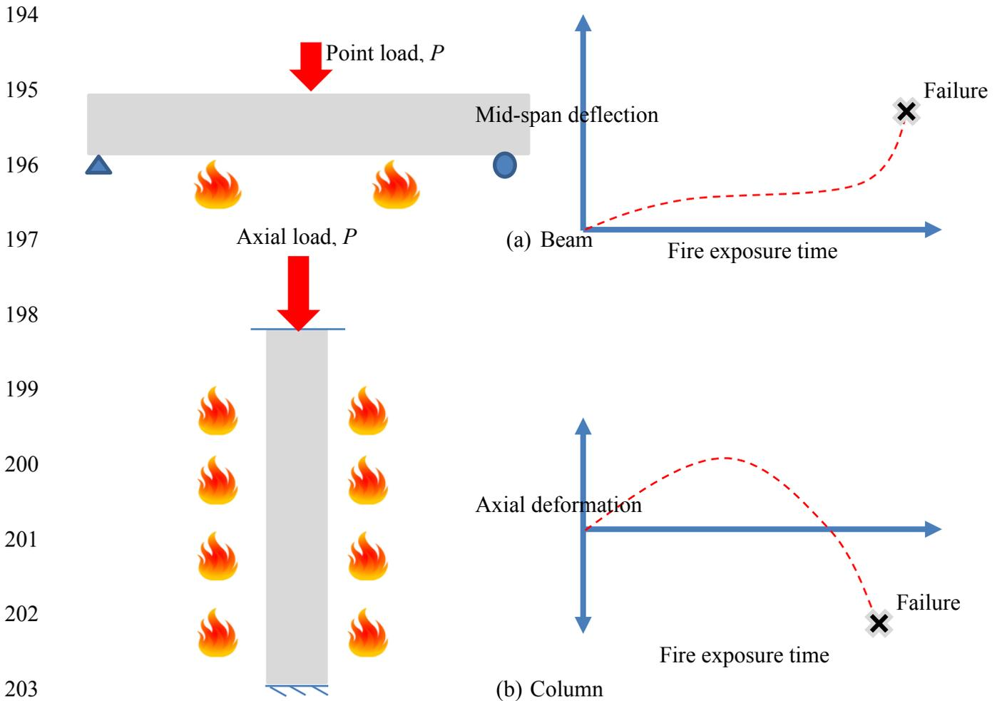
Fig. 3 Typical response of RC beams and columns under fire conditions
