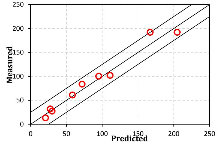
(b) Residual moment capacity of beams (in kN.m)
